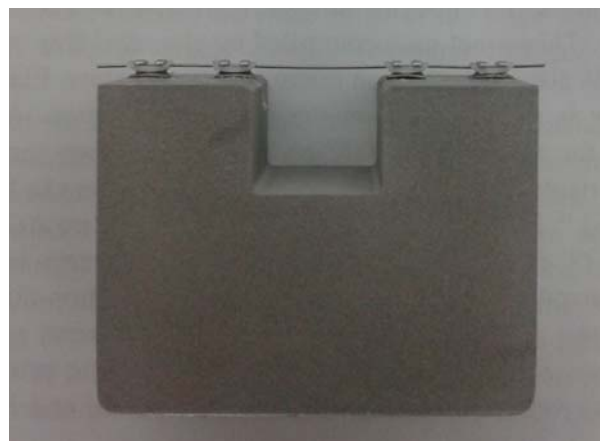
Fig. 2. Three point bending set-up for the load - deflection measurement
